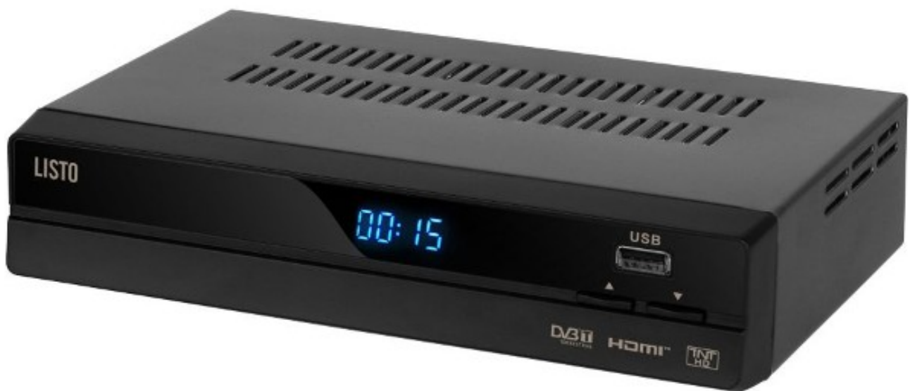
DVB-T device with a USB port ( PVR function ), 30 euros on average
